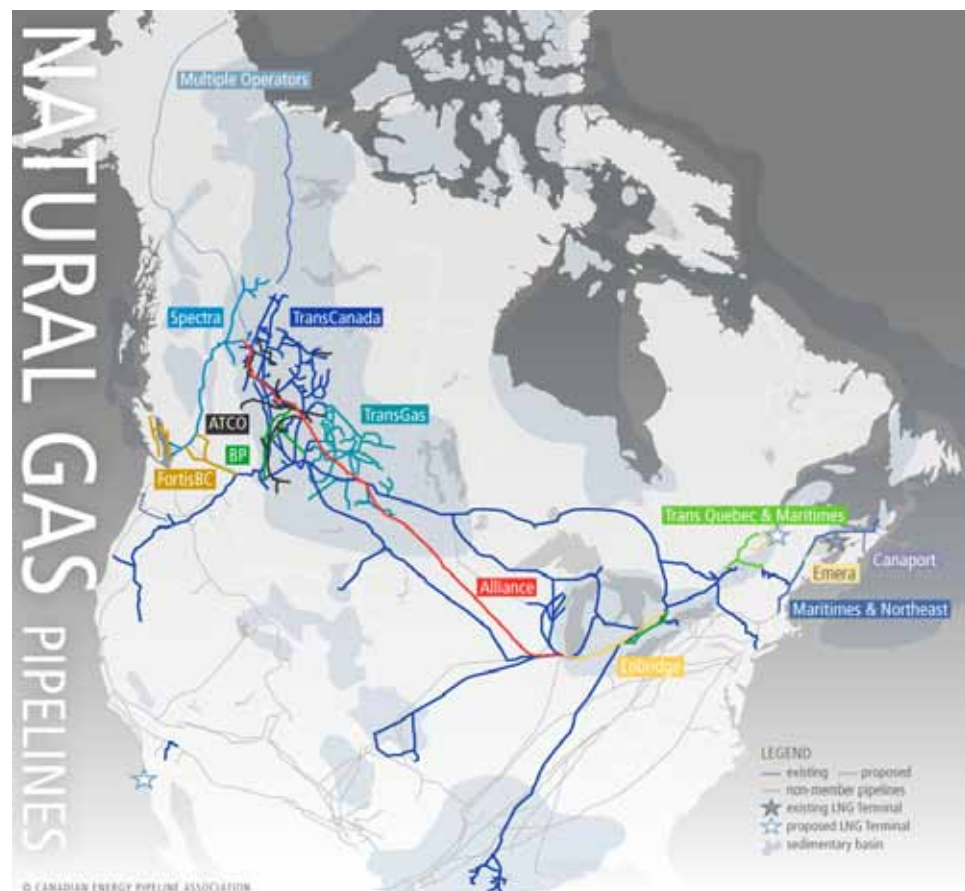
Figure 2 Natural Gas Pipelines
